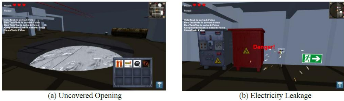
Figure 12. Designed Hazards on the Virtual Construction Site
